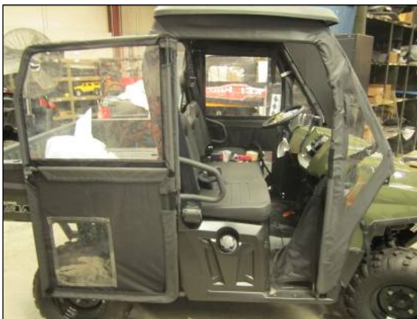
14. Mount the doors by guiding the pins in the back of the door frame onto the hinge barrels along the Rear Hangar Bar.
