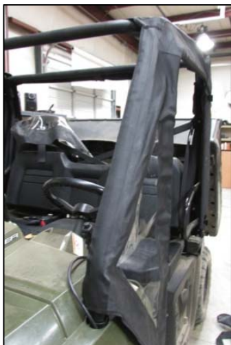
16. Secure side panels to roll cage bars with Velcro. Adjust position as necessary.
